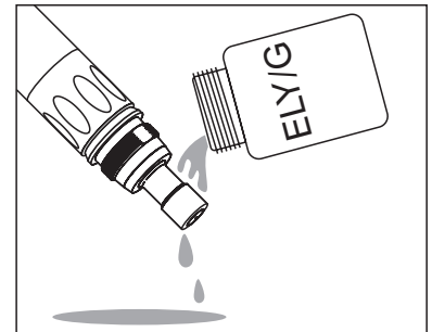
Rinse the sensor head with electrolyte solution.
