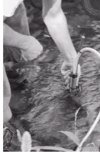
In a stream, the pickup strainer should be submerged under water.
