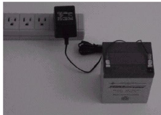
To recharge the battery, fasten the charger's disconnects onto the battery terminals and plug the charger into a wall socket.
