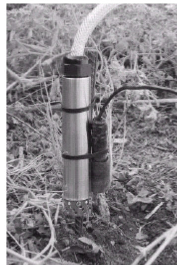
In a dry channel, the rain sensor should be tied just above the debris strainer.
