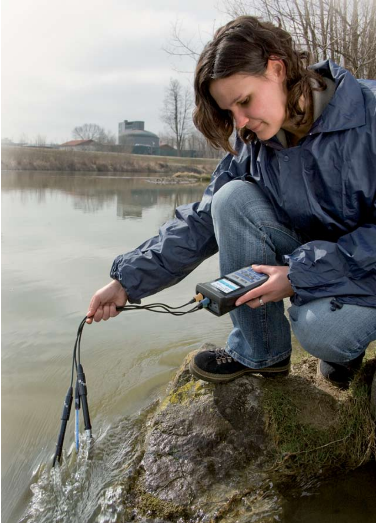
River monitoring using the Multi 3430 Digital Multiparameter Meter with FDO, conductivity, and pH sensors.
